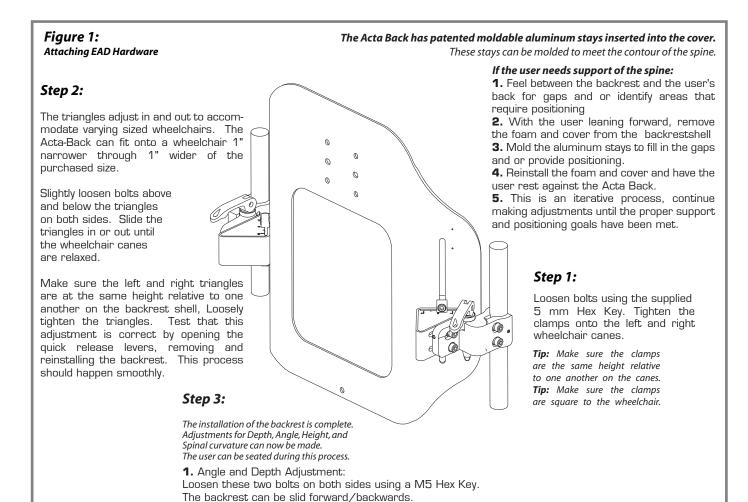
Once backrest is installed onto the wheelchair, other adjustments for height, angle, and depth can be made.
